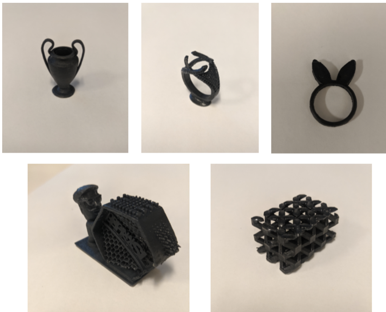
Fig. S4 3D printed objects made with 1:0.9:0.1 (10 mol%) HDT-DAT-TAT: trophy (23.4 mm tall, 1.5 mm thick ears); solitaire ring setting (28.6 mm tall, 1.6 mm thickness ring support); bunny ring (20.4 mm ring size, 12.5 mm ear height); original Prusa SL1 test object (37 mm person height, 2 mm small hexagon size); lattice (27.3 mm width, 40.0 mm length, 25.0 mm height, 3.3 mm support thickness).
