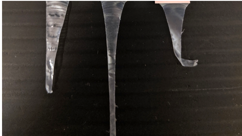
Fig. S2 Dogbones with varying amounts of the crosslinker TAT were elongated to break. During plastic deformation, striations appeared on the dogbone that coincided with dips in the stress-strain profile. Striation appearance decreased with increasing crosslinking density and was in agreement with the decreasing frequency and intensity of the stress dips observed on the stress-strain profile.
