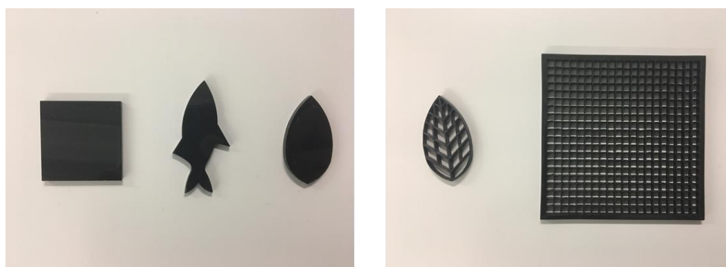
Figure S5. Photographs of Delrin® mold (left) and Delrin® gel cutting grids (right) used in this paper.
