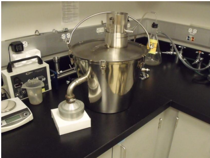
Figure E2. Custom-built Soil Aerosolization Chamber (SAC) for generation and collection of soil aerosols prior to primary plating.
