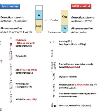
(see below) and chromatographic conditions, e.g. by using toluene in the reconstitution solvent mixture to ensure that very lipophilic components like CE and TAGs are efficiently transferred to the UHPLC column in the injection process.
