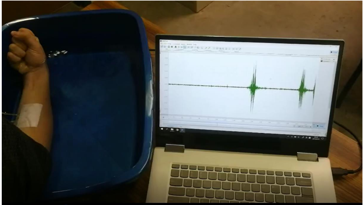
Fig. S22. EMGs recording in water, showing the uncompromised signal quality. Since the Ag NWs side is laminated onto human skin, the conformal contact between the porous SEBS substrate and skin allows the encapsulation of Ag NWs, blocking their direct contact with water, thus providing the waterproof capability of the Ag NWs even in water.
