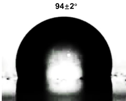
Fig. S6. Water contact angle measurement of nonporous SEBS, showing around 31° lower than that of porous SEBS. The enhanced hydrophobicity can be attributed to significantly increased surface roughness stemming from the porous structures. On a rough surface, water contact angle can be described with Wenzel equation
