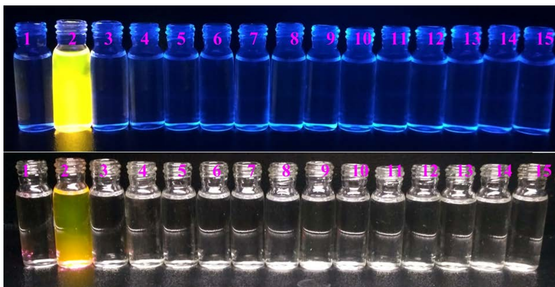
Figure S58. Visual colour changes of chemosensor \text{H}_3\text{L}_3 ( 10\mu\text{M} ) in presence of common metal ions (1equivalent) in 10 mM HEPES buffer (pH 7.4). The images in below row and above row were taken under visible light and UV light respectively. Where 1= only \text{H}_3\text{L}_3 , 2-15= \text{H}_3\text{L}_3 + different metal ions ( \text{Al}^{3+} , \text{Cu}^{2+} , \text{Cd}^{2+} , \text{Pb}^{2+} , \text{Hg}^{2+} , \text{Mn}^{2+} , \text{Fe}^{3+} , \text{Co}^{2+} , \text{Ni}^{2+} , \text{K}^+ , \text{Na}^+ , \text{Mg}^{2+} , \text{Ca}^{2+} and \text{Zn}^{2+} respectively).
