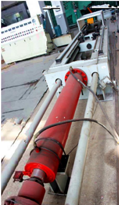
21 Fig 4. Apparatus for the pull-out test and test materials.
