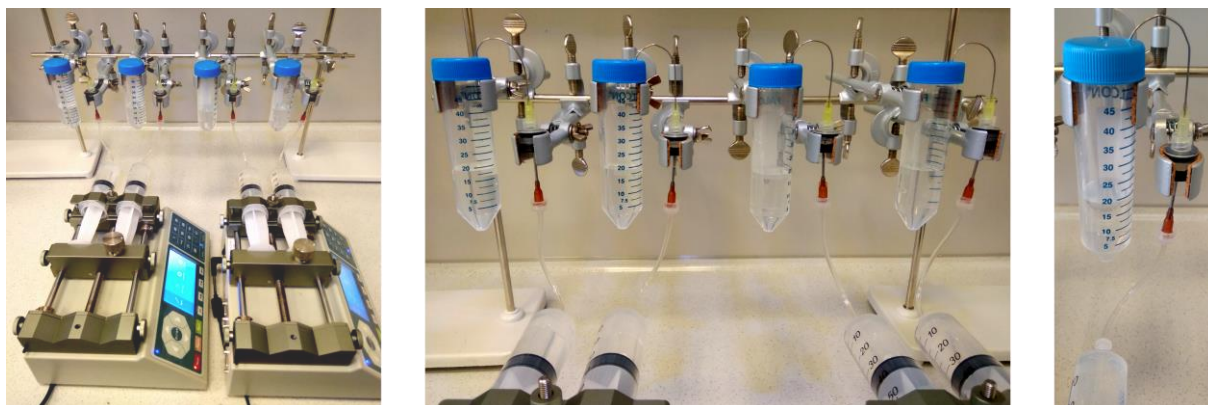
Supplementary Figure 8: Flow reactor set up of four parallel reactors for the production of 4-vinylphenol.
