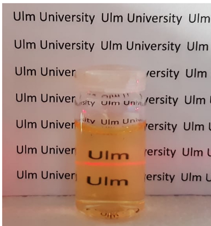
Figure S1. Tyndall effect observed in the solution of K,Na-PHI nanoparticles
