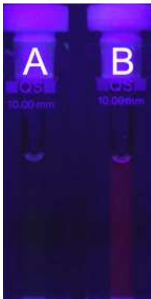
Figure S5. Fluorescence colors of 8b ( c_L = 10 \mu\text{M} ) in the absence (A) and in the presence (B) of ct DNA ( c_{\text{DNA}} = 300 \mu\text{M} ); \lambda_{\text{ex}} = 366 \text{ nm} . The contrast and brightness were enhanced by 30% without changing the true colors.
