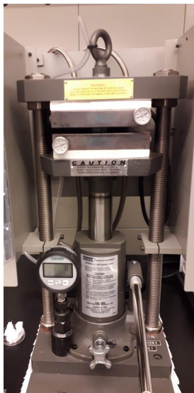
Figure S2. Thermo-compression tool used to bond the PMMA layers in the microfluidics device with the applied bonding recipe.
