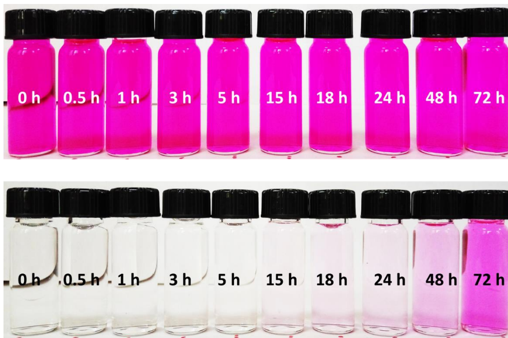
Supplementary Fig. 39 Digital photographs of rhodamine B aqueous solution before and after filtration through FS-COM-1-VF at different times.
