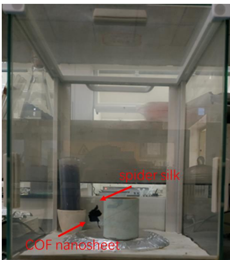
Supplementary Fig. 27 The light-driven experiment which was carried out in a closed balance and COF nanosheet and capillary tube were linked by spider silk in the experiment.
