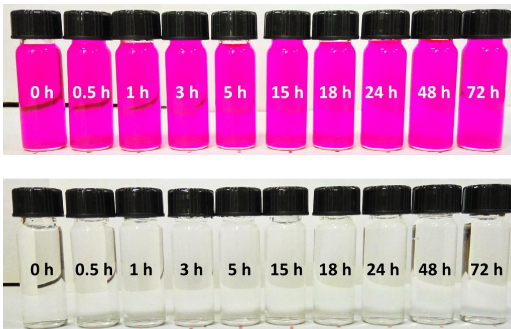
Supplementary Fig. 30 Digital photographs of rhodamine B aqueous solution before and after filtration through FS-COM-1 at different times.
