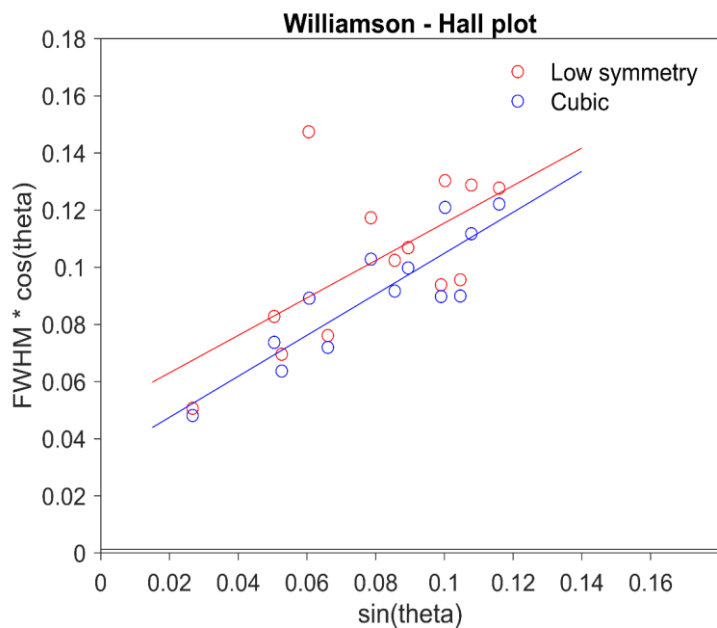
Supplementary Figure 34: Williamson-Hall plot using the peak shape parameter values from the 23 peaks obtained after fitting the two diffraction patterns of interest. Theta values in degrees (°).
