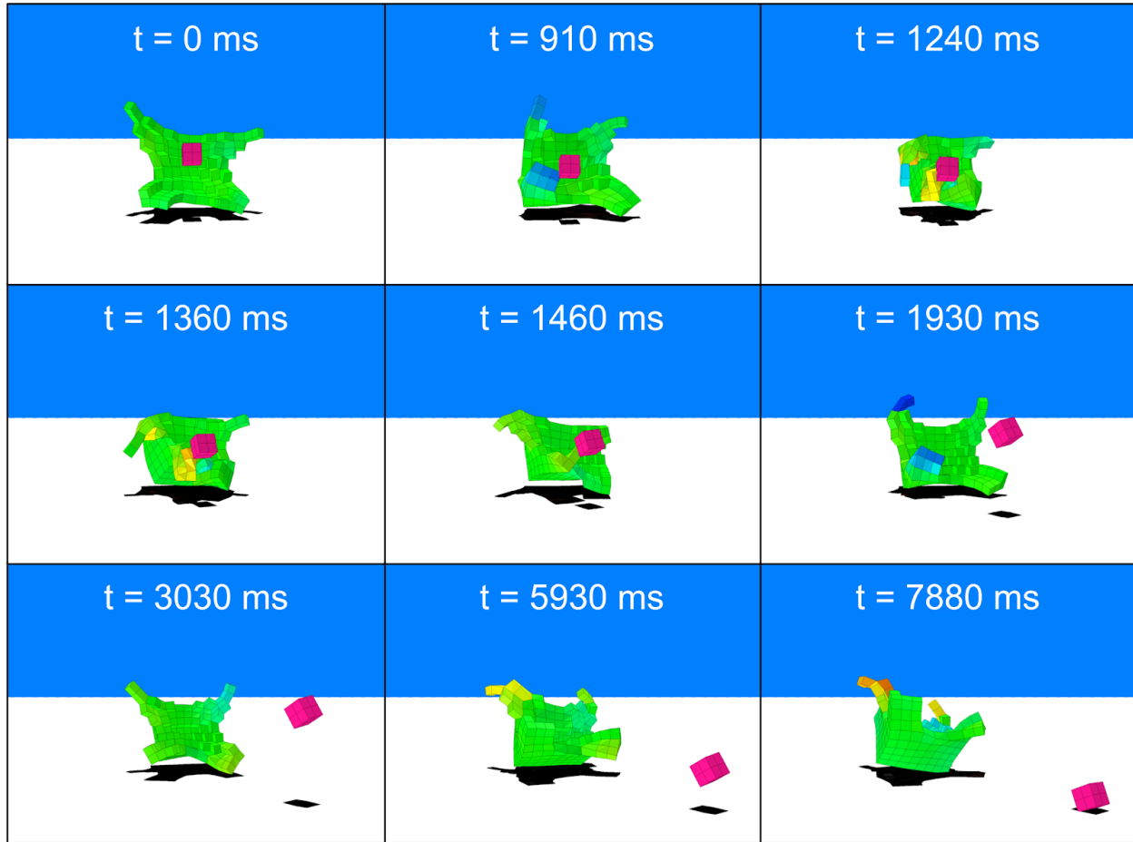
Fig. S14. Object expulsion in silico . A non-locomotion-based goal was supplied to the pipeline: thrown object distance (48). Using an additional objective that maximizes surface-area to volume ratio, limbs evolved which were used to throw a pink 2 \times 2 \times 2 object. For visibility, the voxels in this figure are colored by their angle relative to the ground plane, where green denotes parallel (angle zero), cooler colors (cyan and blue) denote voxel rotations into the right hand side (more or less) of the frame up to -\pi , and warmer colors (yellow, orange and red) denote voxel rotations into the left hand side up to +\pi . The run 2 champion (seed=2) at the end of 1000 generations is pictured. However, this design relies on finely-tuned actuation (which is unlikely to transfer) and fails to pass through the build filter because it is 100% muscle.
