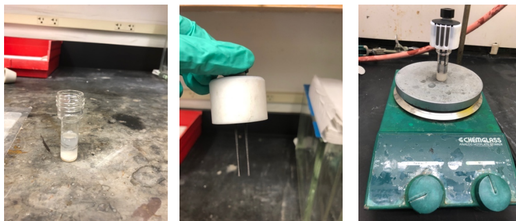
Left: after adding \text{CH}_2\text{Cl}_2 to the vial. Center: graphite electrodes. Right: pre-stir for 15 min.
