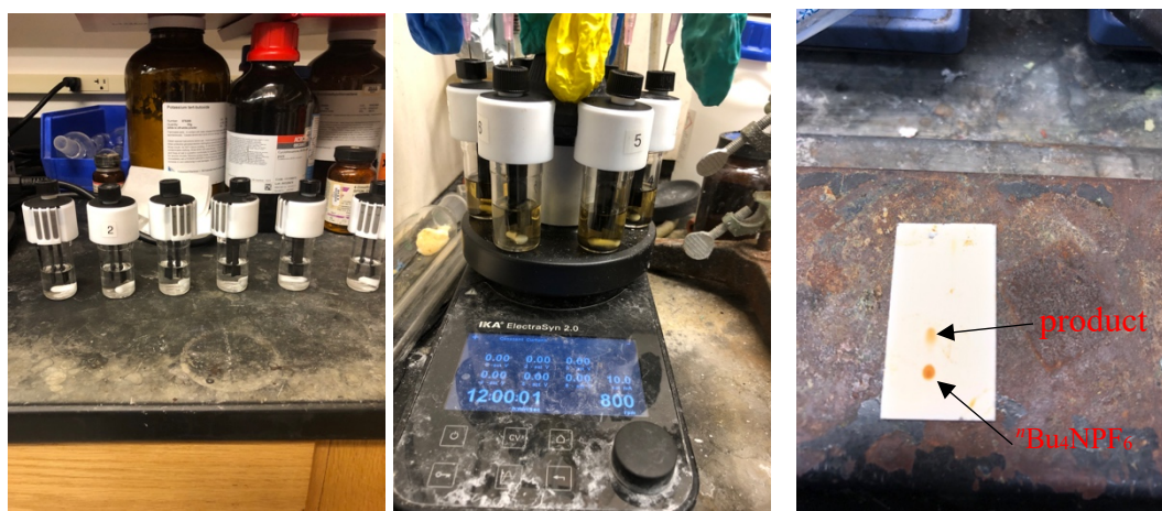
Left: after adding solvent and \text{H}_2\text{O} , and equipped with graphite electrodes. Center: reaction completed (12h). Right: crude TLC (Hexanes: EtOAc= 4:1).
