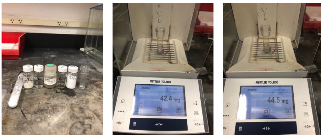
Left: all reagents for this reaction. Center: carboxylic acid (42.4 mg). Right: t -BuOH (44.4 mg).
