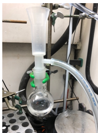
Left: dilute with Et 2 O (30 mL) and washed with sat. NH 4 Cl (aq). Center: washed with brine. Right: dried over Na 2 SO 4 and filtered.
