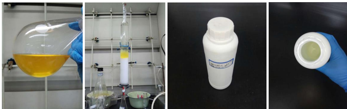
Left to right: crude product, basic alumina chromatography, pure product (bottom and product)
