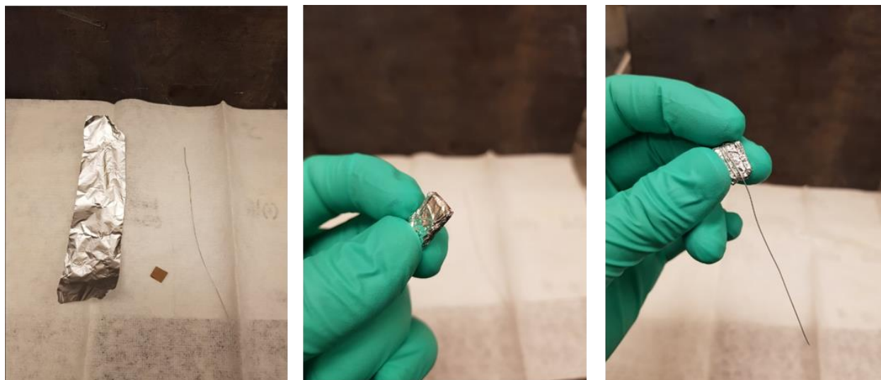
(Left) Al foil, piece of cardboard and galvanized steel wire needed for the cathode for a room temperature reaction. (Center) Wrap the foil over the piece of cardboard. (Right) Wind the wire over this piece several times.
