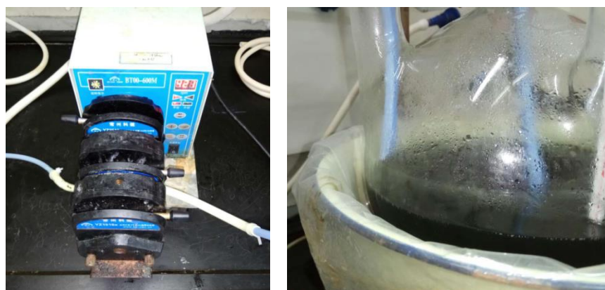
(Left) Peristaltic pump and fluororubber tube. (Right) External round bottom in flow.
