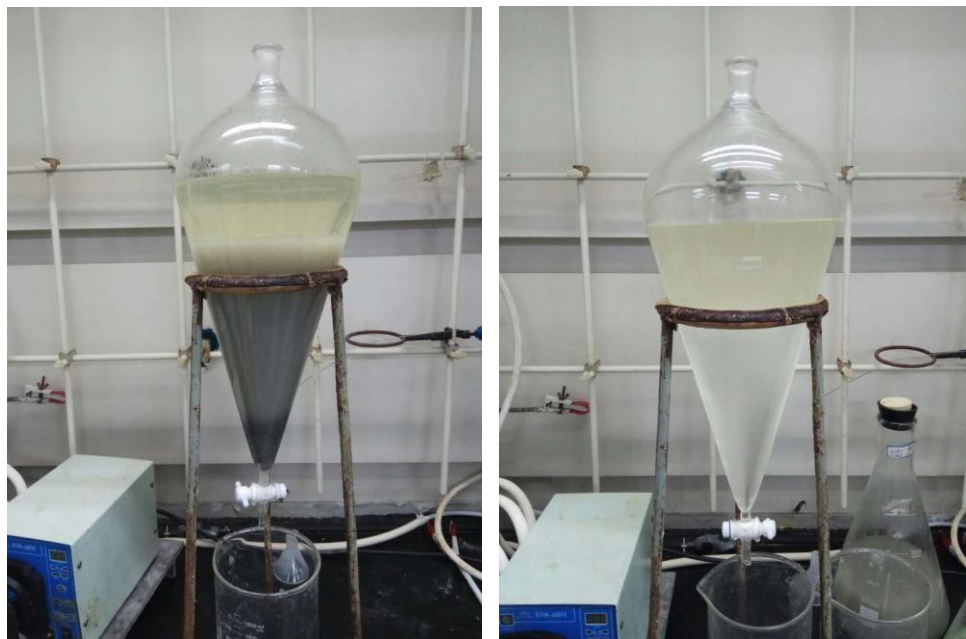
(Left) Reaction mixture washes with 10% Roschelles' salt solution. (Right) Reaction mixture washes with water.
