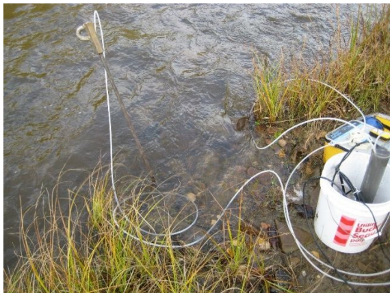
Figure S2 – Photos of shallow groundwater sampling at the edge of the Athabasca River or one of its tributaries away from any tailings pond (i.e., background samples) using the mini-profiler system.
