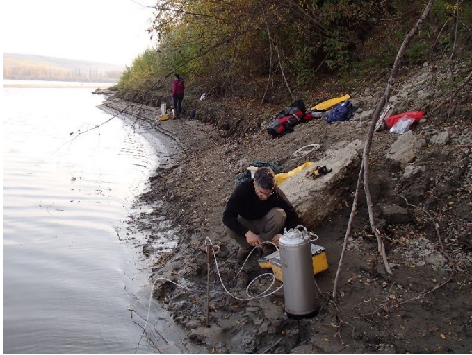
Figure S1 – Photos of shallow groundwater sampling at the edge of the Athabasca River, adjacent to Tar Island Dyke (Pond 1), using the mini-profiler system.
