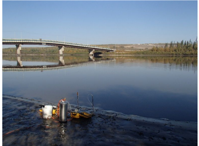
Figure S1 – Photos of shallow groundwater sampling at the edge of the Athabasca River, adjacent to Tar Island Dyke (Pond 1), using the mini-profiler system.
