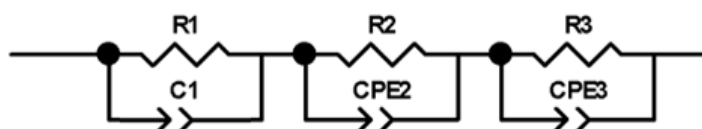
Figure S4. Schematic of the equivalent circuit composed of a series of three resistors and constant-phase elements in parallel to account for the bulk (R1), grain boundary (R2) and interface (R3) resistances present within the cell was used to fit EIS data.
