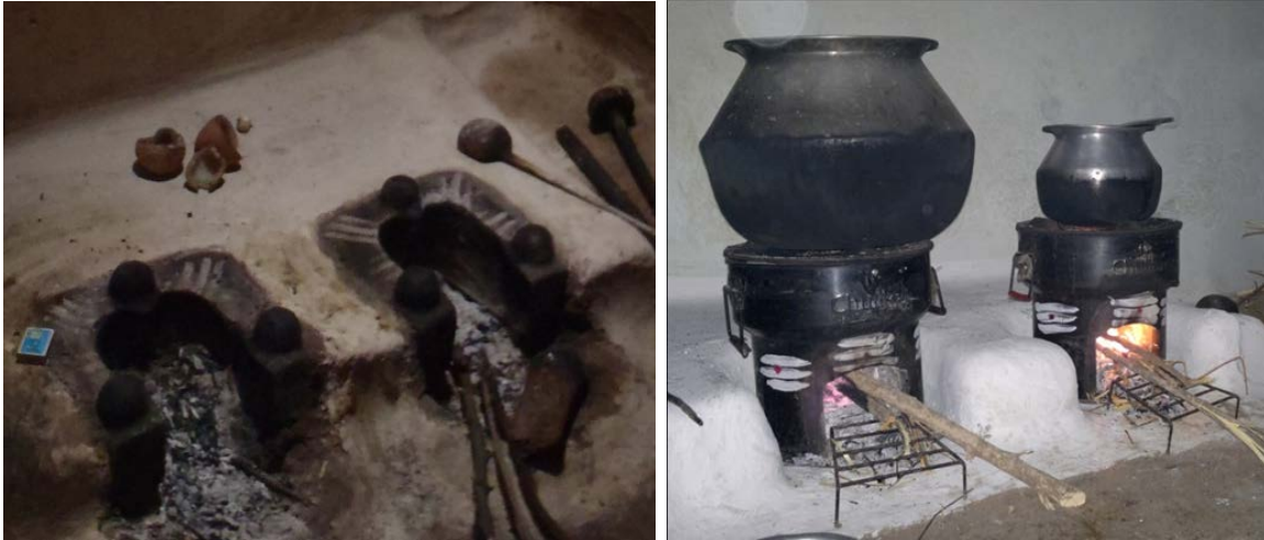
Fig. S1: Photos of traditional chulhas (left) and intervention natural draft 'rocket' stoves (right) assessed in the study.
