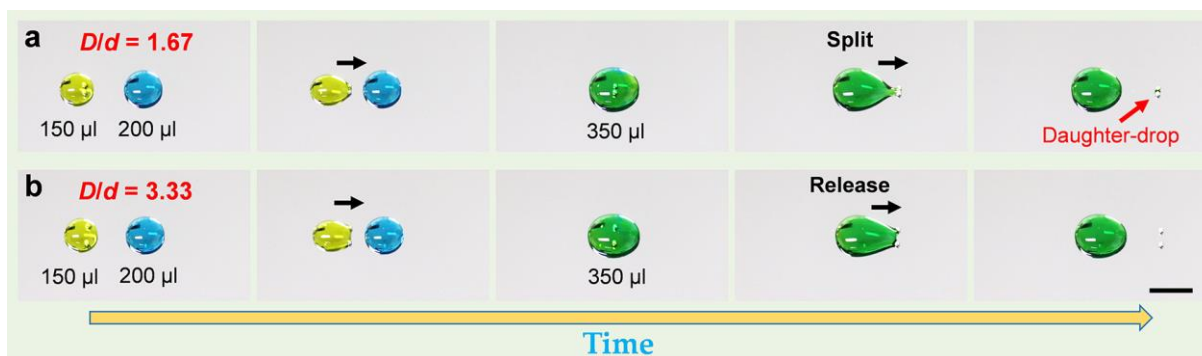
Fig. S4. Demonstration of the droplet behaviors influenced by D/d and V . (A) Manipulation of droplets by the magnetic-actuated with D/d of 1.67. The robot transports a 150 \mu\text{l} droplet to a 200 \mu\text{l} droplet. Then, a daughter-drop is split from the mixing droplet. (B) Manipulation of droplets by the magnetic-actuated robot with D/d of 3.33. The robot releases the mixing droplet after transport a 150 \mu\text{l} droplet to a 200 \mu\text{l} droplet. The black arrows indicate the moving directions of the robot. The moving speed is 2mm/s. Scale bar, 10 mm.
