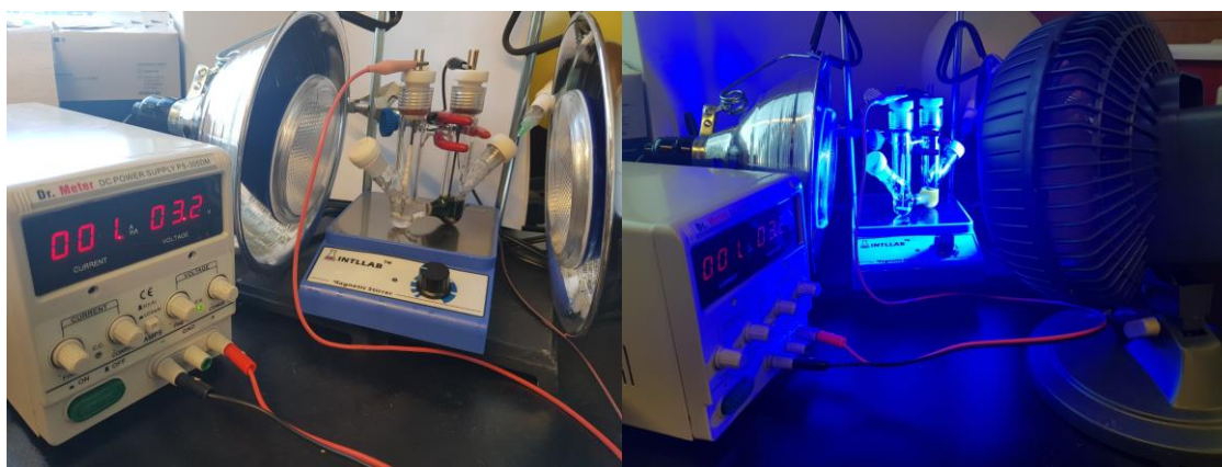
Figure S2. Setup for Reductive Electrophotocatalysis: Before Light On (Left), After Light On (Right)
