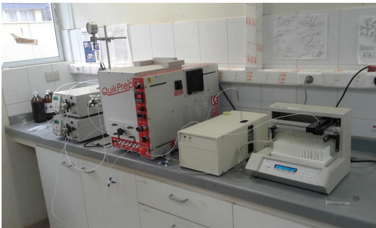
Figure S1. Quattro MK-7 HSCCC system, equipped with two HPLC pumps, UV detector and fraction collector.
