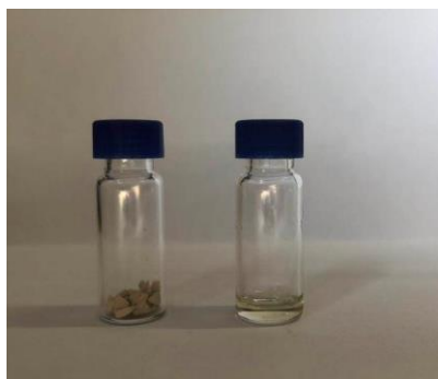
Figure S18. Images of PE with ester units in the backbone before (left) and after (right) degradation, related to Figure 5.
