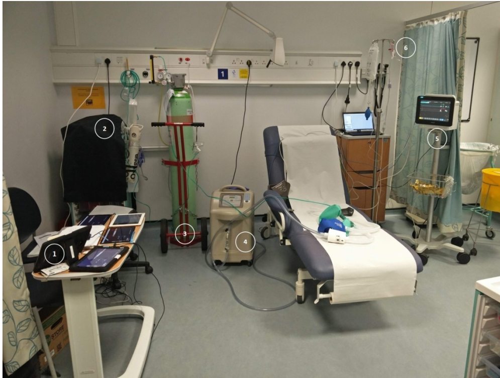
Figure 2: Hypoxia study day set up. Legend: 1- Tablets linked with AMD devices (4 Samsung Tab A, each linked with one AMD: AP-20, WristOX2 3150 BLE, CheckMe O2 and VitalPatch®. 1 iPad 4 connected to the Wavelet). 2- Resuscitation trolley and Oxygen. 3- 7% oxygen in nitrogen cylinder. 4- Hypoxicator apparatus. 5- Philips monitor (model MX450) connected to laptop (IX Trend software). 6- Drip stand with the arterial line pressure bag.
