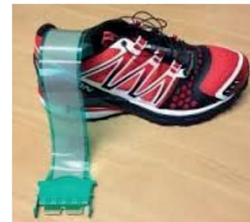
This entails using electronic insoles inserted into the patients current footwear which provides readouts of varying pressures under the soles of the feet as shown below.
