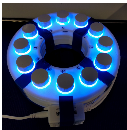
Figure S6: 3D printed light reactor equipped with LED strips. Left: 3D concept of light reactor, made with autocad. Right: Final 3d printed light reactor holding 20 mL vials and lined with led strips
