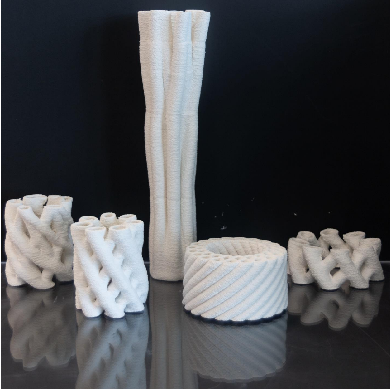
Supplementary Figure 4 | Additional examples of geometries 3D printed with FLAM and unable to be produced by traditional casting or molding techniques.
