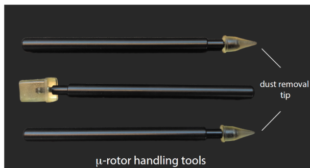
Figure S3. \mu -rotor handling tools. The rubber tips help in removing the residual particles on the \mu -rotor and caps surfaces (dry residues, dust, etc.).
