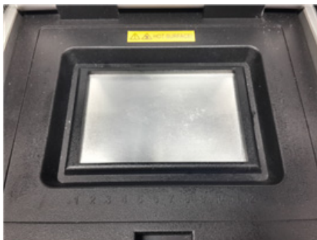
Figure S2. A tailor-made flat heat block was used to conduct chip-based PCR, instead of using conventional heat block which contains either 48 or 96 wells to hold PCR tubes,
