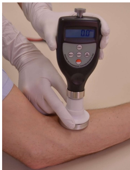
Durometer, zero'ed and inserted into skin conditioning ring.
