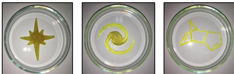
Pictures of more sophisticated patterns made of poly(dicyclopentadiene 12 ) in 80 mm x 15 mm petri dishes.
