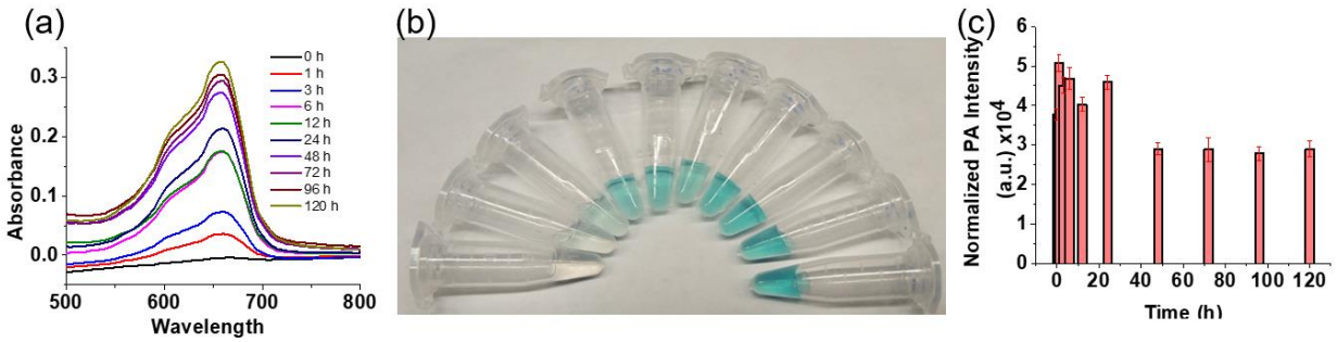
Figure S10. (a) Absorbance of supernatants collected during the drug release study of PLGA NPs loaded with PTX-LMB in PBS with 20 % mouse serum at 0, 1, 3, 6, 12, 24, 48, 72, 96, and 120 hours. (b) photograph of the aliquots collected corresponding to the absorbance in (a). (c) the particles isolated from each aliquots were dispersed in 1% agarose to avoid precipitation (leading to small variations in photoacoustic signal) and 3D image of the dispersions were acquired after the allowing the dispersion to solidify. (c) shows that the photoacoustic intensity of the isolated particles did not follow a specific trend. This is in contrast to the photoacoustic signal of the supernatants of the aliquots.
