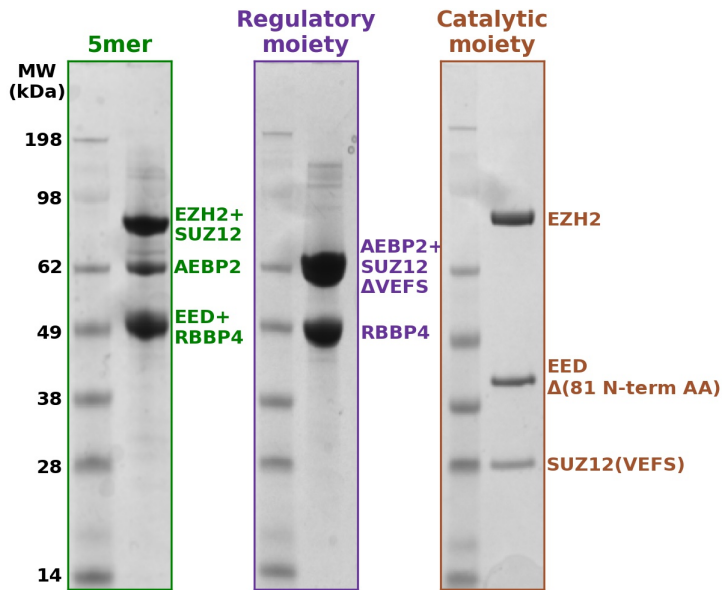
Figure S1. Polyacrylamide gel electrophoresis (PAGE) demonstrates purity of PRC2 moieties. From left to right, PAGE results are shown for the full complex (green text), regulatory moiety (purple text) and catalytic moiety (brown text). For each PRC2 variant, the same ladder is shown on the left lane, and the right lane depicts the PRC2 variant. The ladder is labelled by the molecular weight in kilodaltons, and the major bands for each PRC2 variant are labelled by their constituent components.
