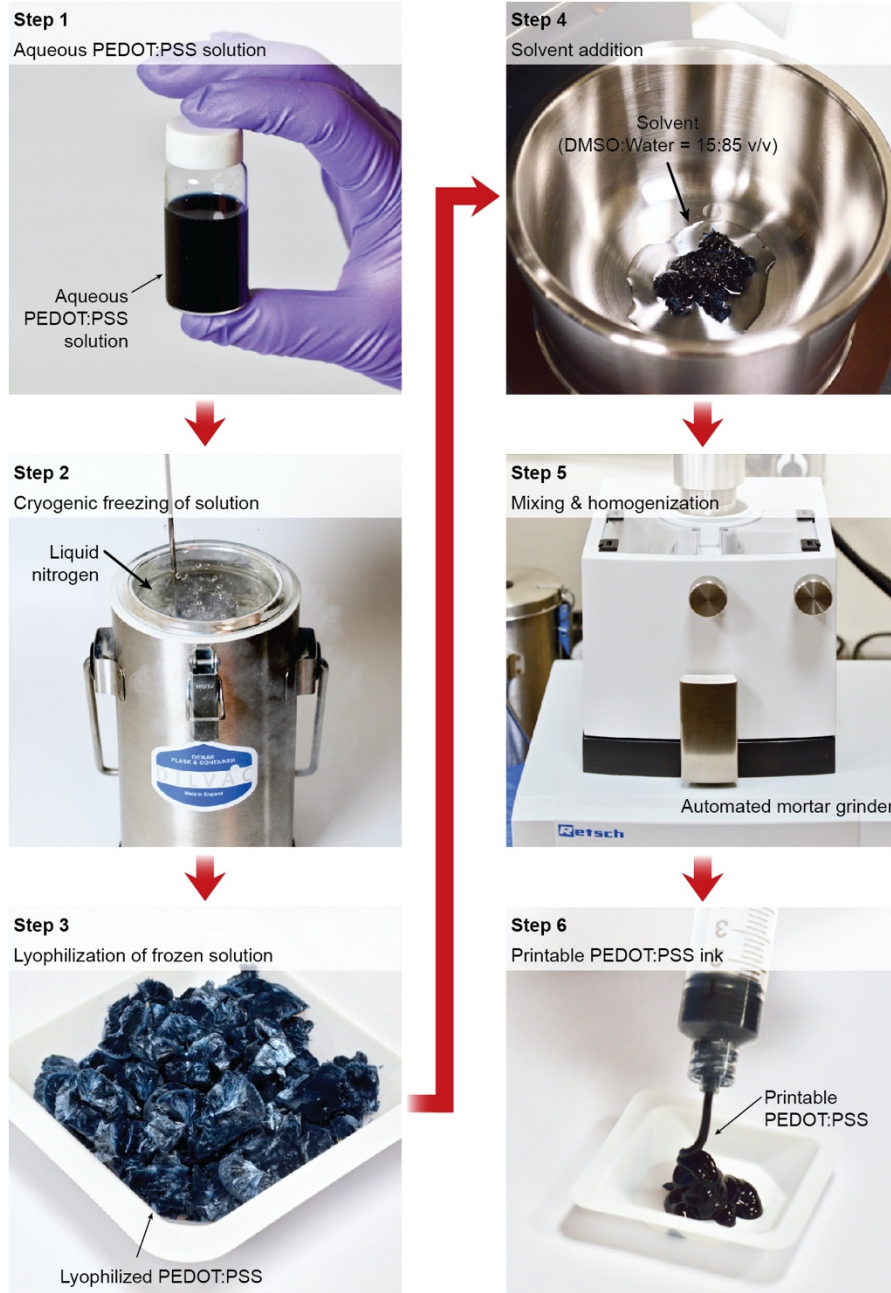
Supplementary Figure 1 | Preparation of 3D printable conducting polymer ink. Step 1, Stirring and filtration of a pristine PEDOT:PSS aqueous solution; Step 2, Cryogenic freezing of the PEDOT:PSS solution in a liquid nitrogen bath; Step 3, Lyophilization of the cryogenically frozen PEDOT:PSS solution to isolate PEDOT:PSS nanofibrils; Step 4, Re-dispersion of the PEDOT:PSS nanofibrils with a solvent mixture (water:DMSO = 85:15 v/v); Step 5, Mixing and homogenization by using a mortar grinder; Step 6, The resultant homogeneous 3D printable conducting polymer ink.
