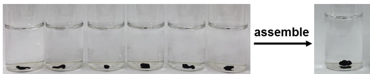
Figure S7. Several as-formed gold hydrogels assemble together into one self-supported hydrogel.
