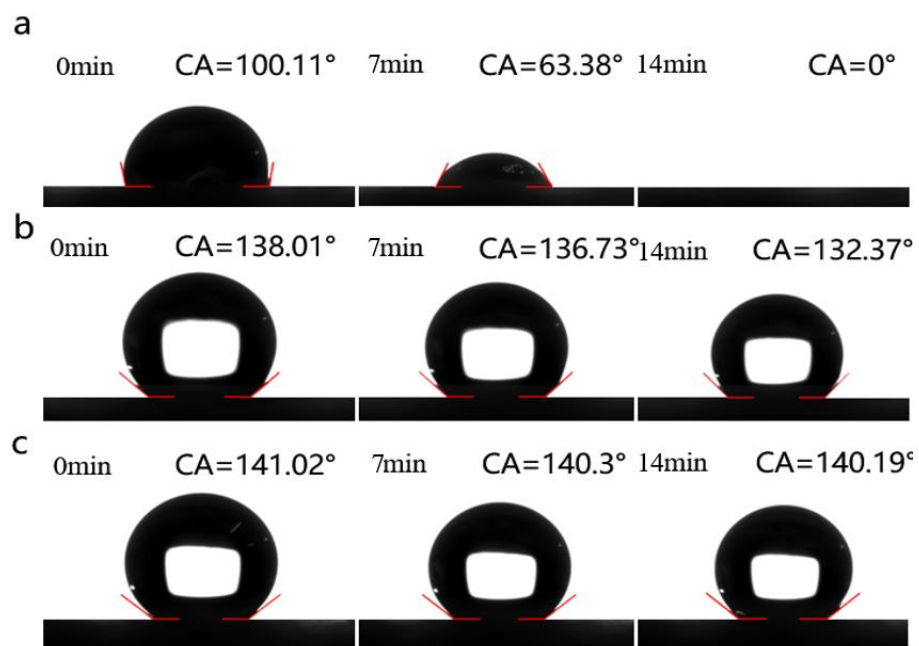
Supplementary Figure 5. Photographs of the contact angle of the catalytic layers as a function of time with (a) PTFE / CB =0.2; (b) PTFE / CB =0.5; (c) PTFE / CB =0.6.
