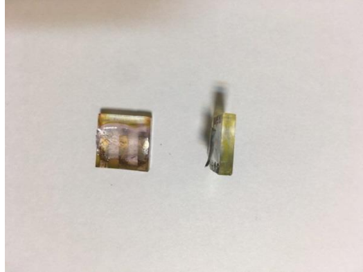
Figure S2 Photo of the damaged device encapsulated by 2:1, PEG: resin ratio system .
