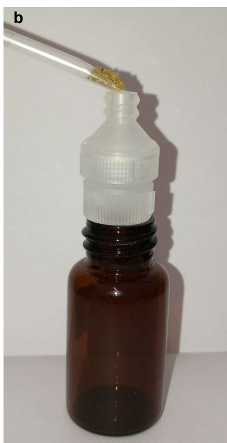
Figure S1. (a) Extraction chamber. A and D, polypropylene disk holder; B, O-ring; and C, Fluoropore™ membrane filter (polytetrafluoroethylene) with a 1.0 \mu\text{m} pore. (b) After the assembly of all parts, sample is placed inside the A moiety, through its wider opening.
