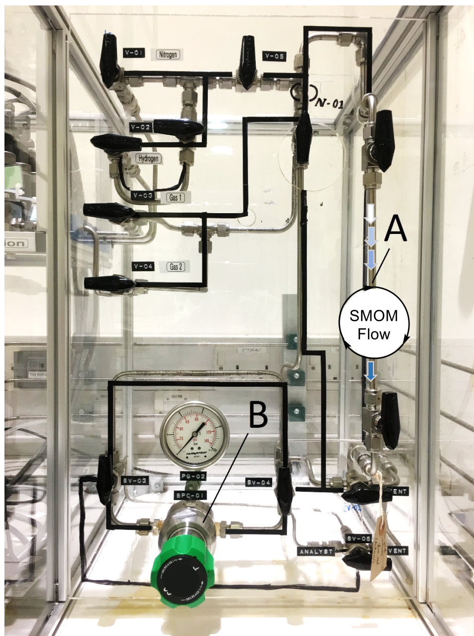
Figure S4: Bespoke continuous gas flow reactor setup fitted with the pre-loaded stainless-steel column (A) containing the catalyst or pre-catalyst, during a catalytic run. Note that the N_2 and H_2 feeds are closed whereas the gas 1 (1-butene) and gas 2 (isobutene) feeds are open and set to pass via the column (A). The outflow is set to pass via the loop, fitted with a regulator (B) to allow H_2 pressurisation, and into the gas chromatograph, 'analyst'.
