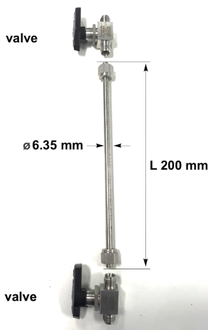
Figure S2: Stainless steel column fitted with gas-tight valves where either the catalyst or pre-catalyst were charged before the catalytic runs under continuous gas flow conditions. This column was fitted to the continuous gas flow reactor using the upper and lower gas-tight two-way Swagelok valves (Figure S4, A).
