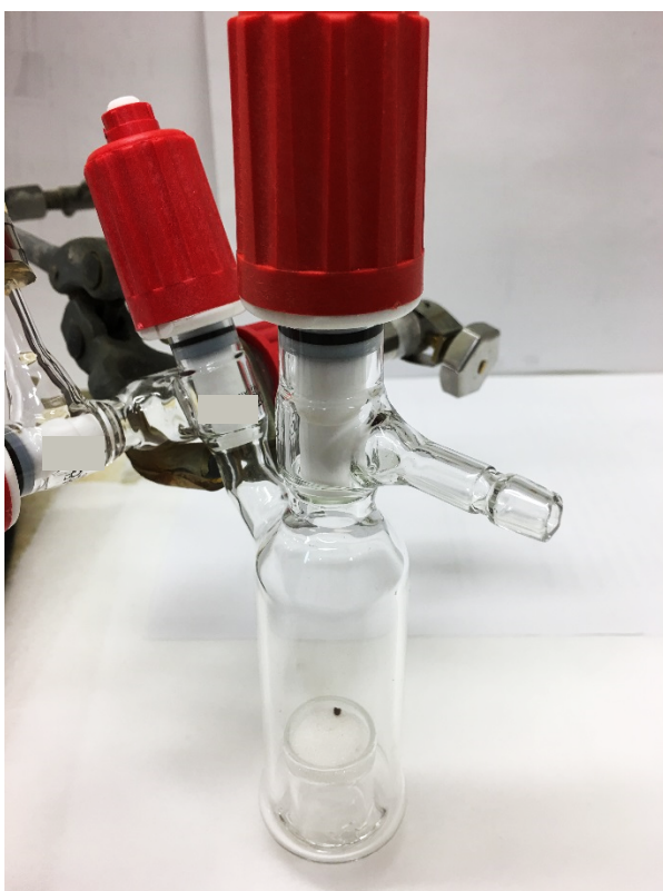
Figure S61: Custom reactor vessel, with high-pressure NMR tube fitted (top), and mounted single-crystal detailed (bottom right).
