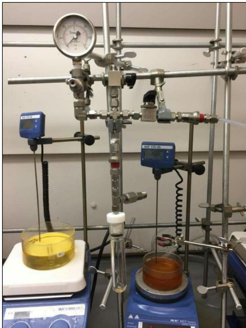
Swagelok setup for pressurizing reactions
