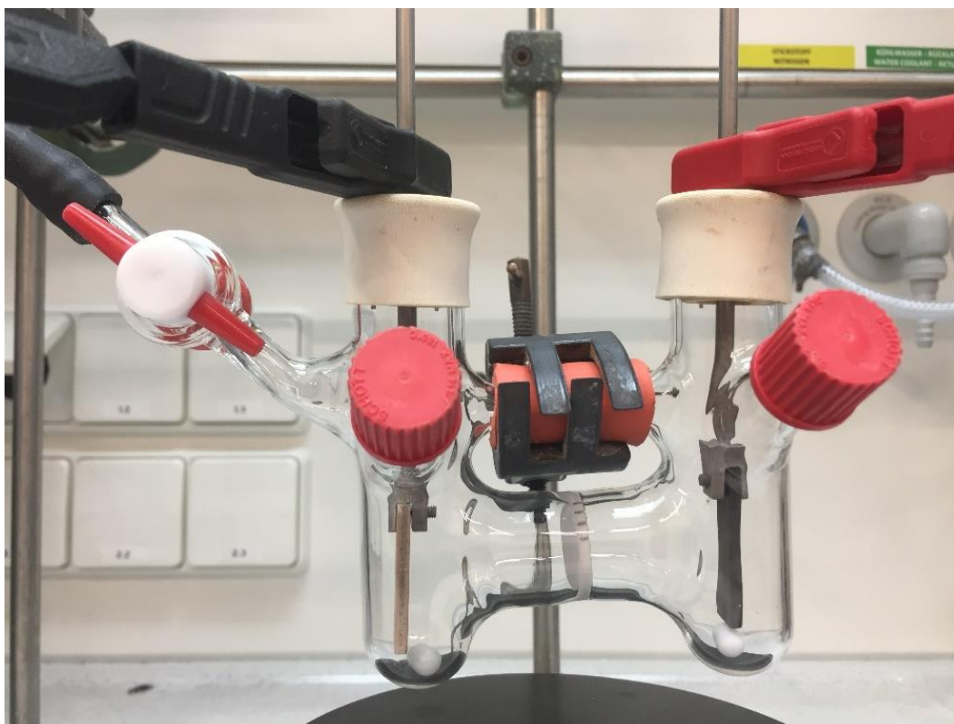
Figure S1. H-type electrolysis cell, divided by a glass frit (G4); left: \text{CuSn}_{17}\text{Pb} cathode; right: graphite anode.
