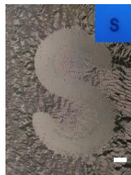
Supplementary Figure 8. LSCM images of “S” wrinkled pattern obtained by “S” mask. Inset picture is corresponding photograph of PDMS taken under UV light.
