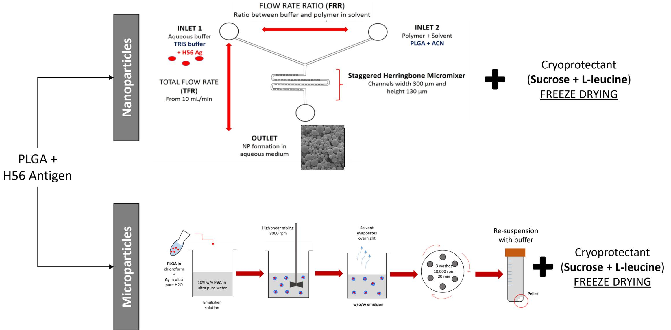
**Figure S1.** Schematic representation of the manufacturing processes for the PLGA nanoparticles and microparticles encapsulating H56 antigen. Nanoparticles were produced using microfluidics at a TFR 10 mL/min and FRR 1:1 whereas microparticles were prepared using the double emulsion method. Cryoprotactants were added post-manufacture and then, particles were freeze dried.
