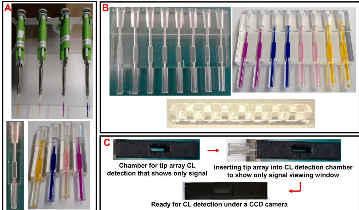
Figure S2. (A) Photographs of the single chamber ELISA in a tip array, as printed and filled with different colored dyes. (B) Multi chamber/ 8 channel ELISA in a tip platform, as printed and colored dye filled showing 4 biomarker detection application. Inset 8 well 3D printed add-on for use in multi analyte analysis. (C) A non-transparent chamber for CL detection that blocks unwanted CL from the sampling conduit and dead volume conduit.
