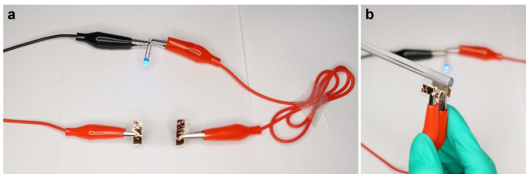
Fig S59. (a) Optical image of CAT-1-on-SLG-25 nm construct on PET substrate at the flat state. (b) Optical image of CAT-1-on-SLG-25 nm construct on PET substrate at the bending state. Bending radius is 3 mm.
