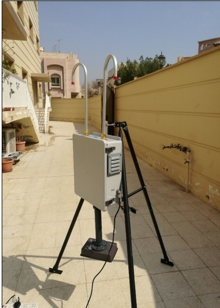
Figure S2: Harvard samplers collecting PM_{10} and PM_{2.5} outside a Kuwaiti home.
