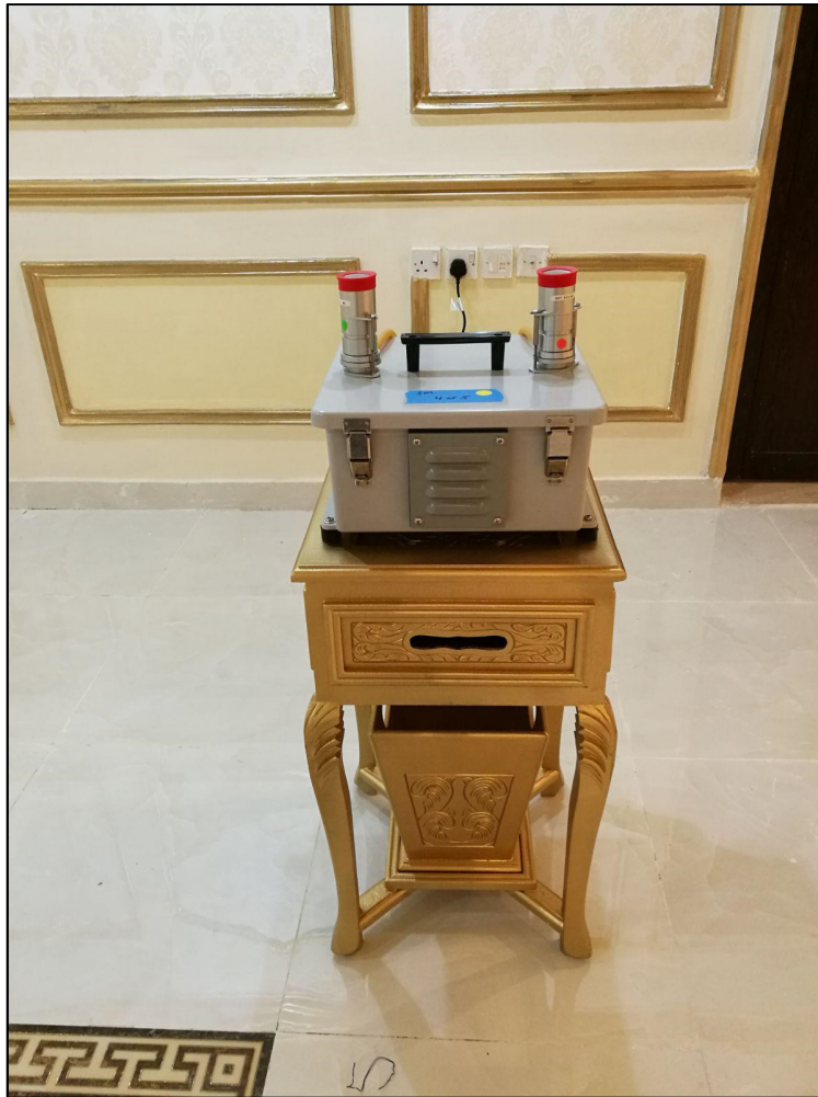
Figure S1: Harvard samplers collecting PM 10 and PM 2.5 inside a Kuwaiti home.
