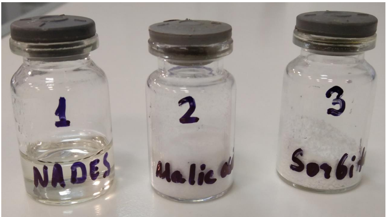
Figure S5: A photo of the physical state of malic acid, sorbitol, and a sorbitol-based NADES (sorbitol : malic acid : water with molar ratio 1:1:3)
