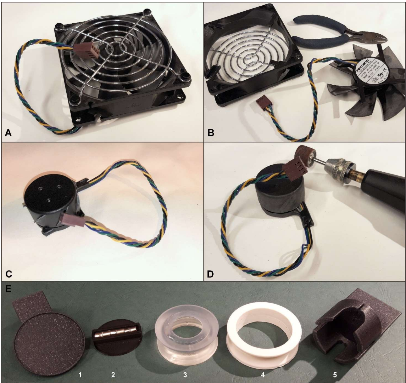
Figure S2. Preparation of a brush-less motor for in-syringe stirring. (A) Use of a computer fan with pulse-width modulation control of velocity, (B) cutting away the supporting frame, (C) breaking off all wings, (D) sanding down excess ends to obtain a smooth surface shell. (E) 3D printed motor attachments for NdFeB magnet placement (E2) or pulley-wheel function (E3, E4) and motor supports as shown in Figures 3 and 4 (E1, E5).
