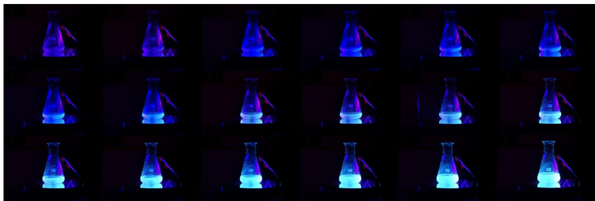
Figure S7. Photographic representation of the viscochromic response of 1 (150 \mu M) in DMSO/glycerol mixtures upon increasing the fraction of glycerol under UV illumination ( \lambda_{exc} = 360 nm). The viscosity of the mixture, and therefore the PL intensity, increase with increasing amount of glycerol added due to aggregation-independent RIM. Top left: DMSO solution of 1; Bottom right: 1 after addition of glycerol to the final ratio DMSO/glycerol = 1:8 mixture.
