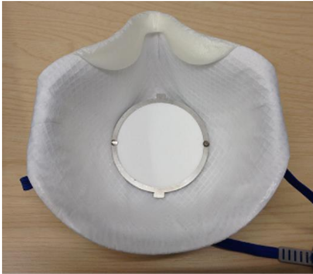
Figure S1: FFP1 face mask containing a gelatine filter with a diameter of 60mm
