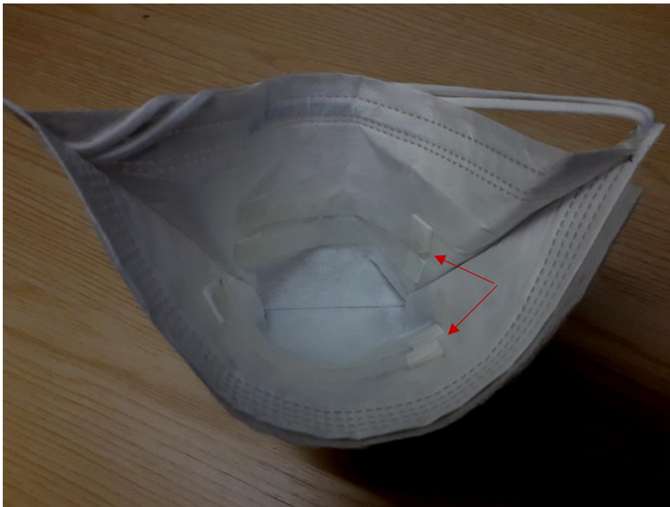
Figure S2: Duckbilled Face Mask containing 4 strips (arrows) of 3D printed Polyvinyl Alcohol (PVA) each measuring 90mm x 10mm.
